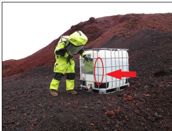
Figure 4: The 250 gallon (946 L) backup tank with graduated measure on the side of the tank highlighted. Photo Credit: Dr. Sian Proctor
