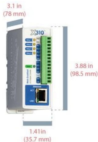
Figure 10: The ControlByWeb X310 Telemetry router
