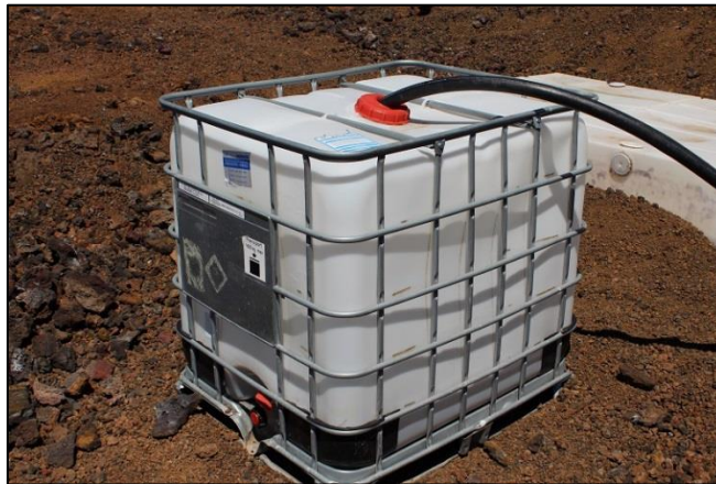
Figure 6 The 250 gallon grey water tank. Measurements were manual using graded markings on side of the tank. Photo Credit: Dr. Sian Proctor
