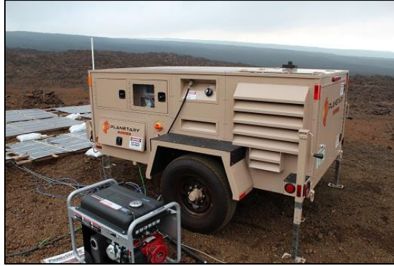
Figure 7: Planetary Power generator seen with the Honda backup generator
